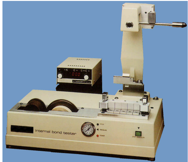
▲ Model 1314 Internal Bond Tester measures the internal bond strength of paper and board.
