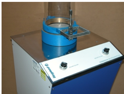
Pneumatic controls for filling, mixing and draining
