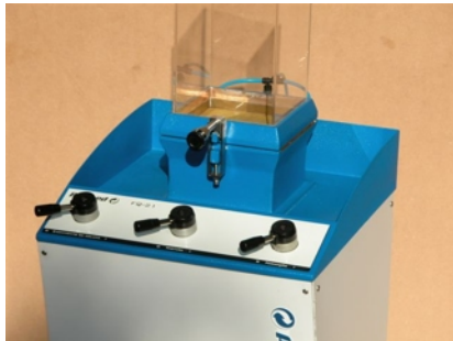
Pneumatic controls for filling, mixing and draining
