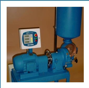
The MD-3000 is a disc refiner widely used for pilot refining of pulps in the Q.C. (quality control) and R&D (research and development) of pulps, papers and boards.
