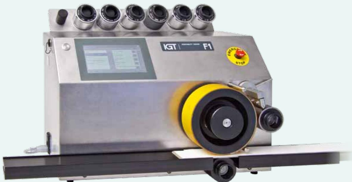
IGT Testing Systems has developed the advanced computerised F1 printability testers for flexo and gravure inks. The F1 makes colour strips with flexo and gravure inks, which can be used for many purposes and has specially been designed to aid computerised colour measuring and colour matching systems. The F1 saves on costs because colour testing on the printing press is no longer necessary.
