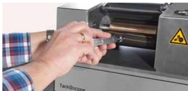
All IGT tack devices are based on three roller systems according to ASTM D 4361 and ISO 12634 with a driver centre roller, a distribution roller (oscillating roller for distribution of the ink) and a measuring roller (connected with the tack sensor).
