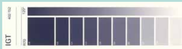
Gravure print to check the colour in ten coverages and/or to check the roughness of the substrate
