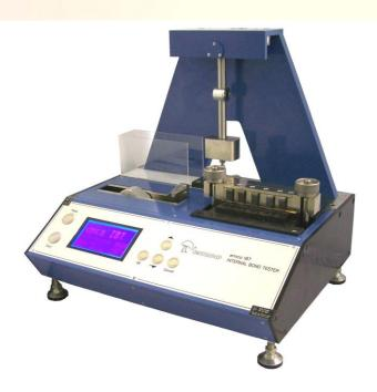
The *emco* **IBT Internal Bond Tester** realize a dynamic measuring principle to determine the internal bond strength of paper, board and compound materials. The significant influences of sample preparation and climatic conditions became consideration in the construction.
