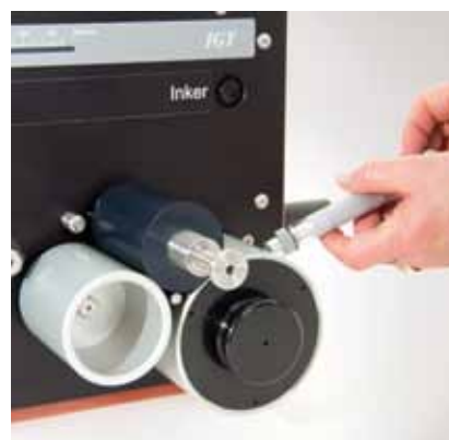
Applying ink with the IGT ink pipette
