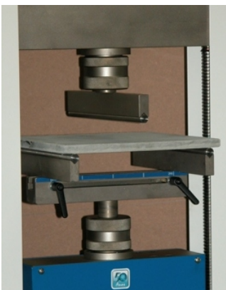
Deflection of plane cement boards
