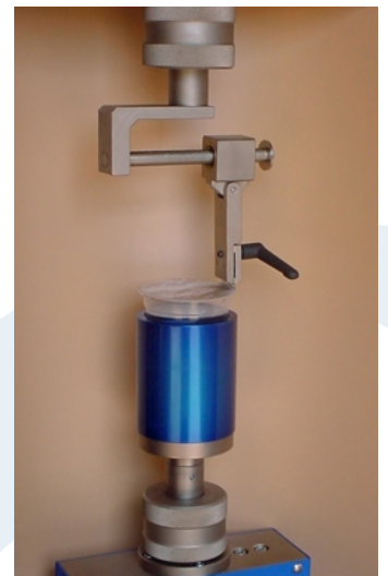
Peel opening force of cups and jars
