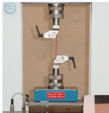
Rupture of wires
