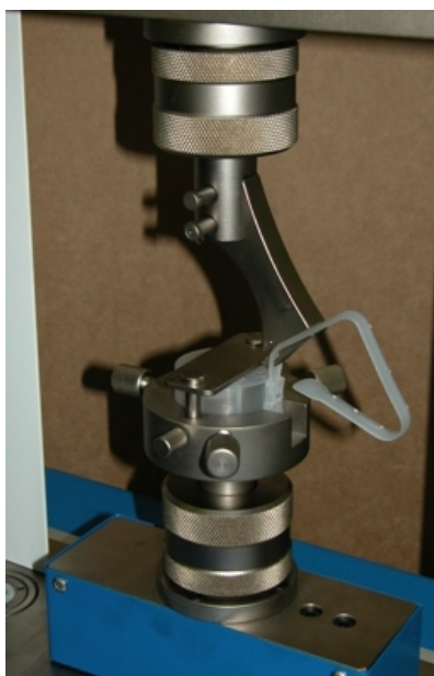
Extraction of plastic fitting
