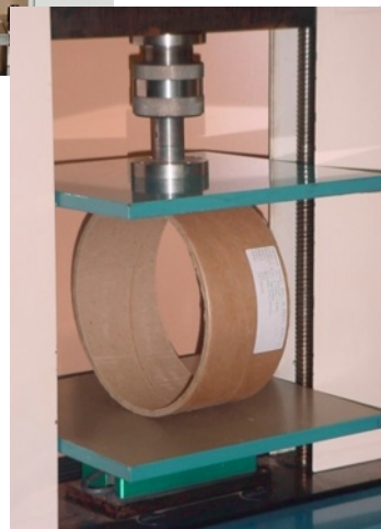
Core compression Applicable standards: ISO 11093-9
