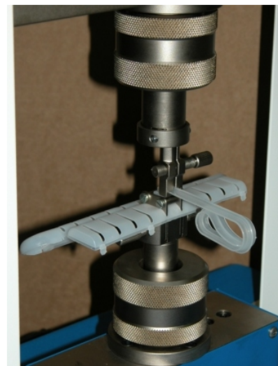
Rupture of plastics packing
