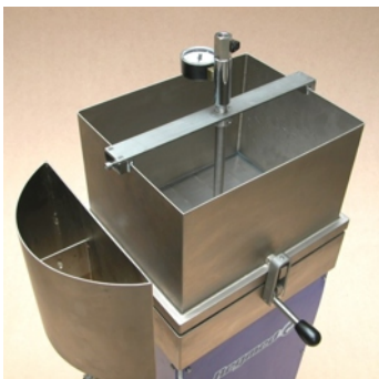
General view of screen box, screen plate, nozzle and weirbox
