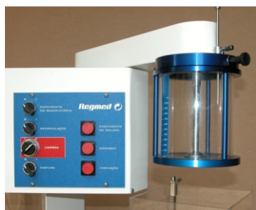
Dosing unit and control panel
