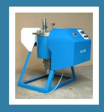
The laboratory reactor model HB-51 has been designed for pilot chemical, semi-chemical and thermal pre-treatments of several types of biomass.
